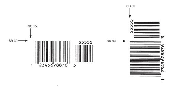
Figure 5-28. Sample UPC-A Bar Codes with Add-On Data
